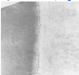
Off-corner internal crack (forms bellow mold, small corner radius)
